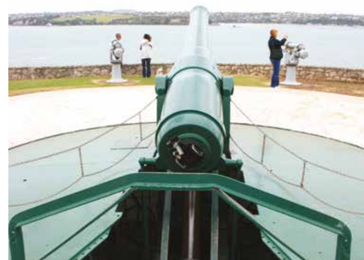
THE LONG ARM OF EMPIRE: An 1886 Armstrong 8 in coastal defence gun on a hydraulic disappearing mounting at North Head, Auckland, New Zealand.
