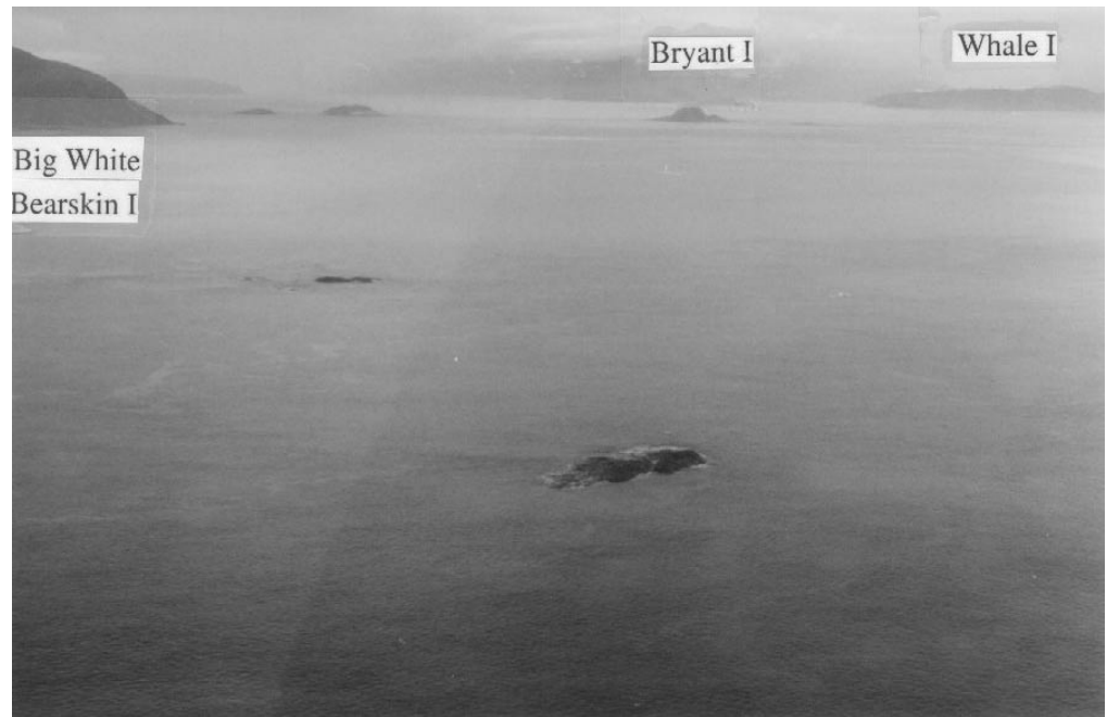
Figure 2. Unnamed rock east of Big White Bearskin Island ( 59^{\circ} 21' 54''\text{N} , 63^{\circ} 25' 22''\text{W} ) as photographed and positioned by GPS in 1997. In 1973, this rock was also positioned by angles and distances of an electronic distance measurement traverse. It is 1.1m above high water.
