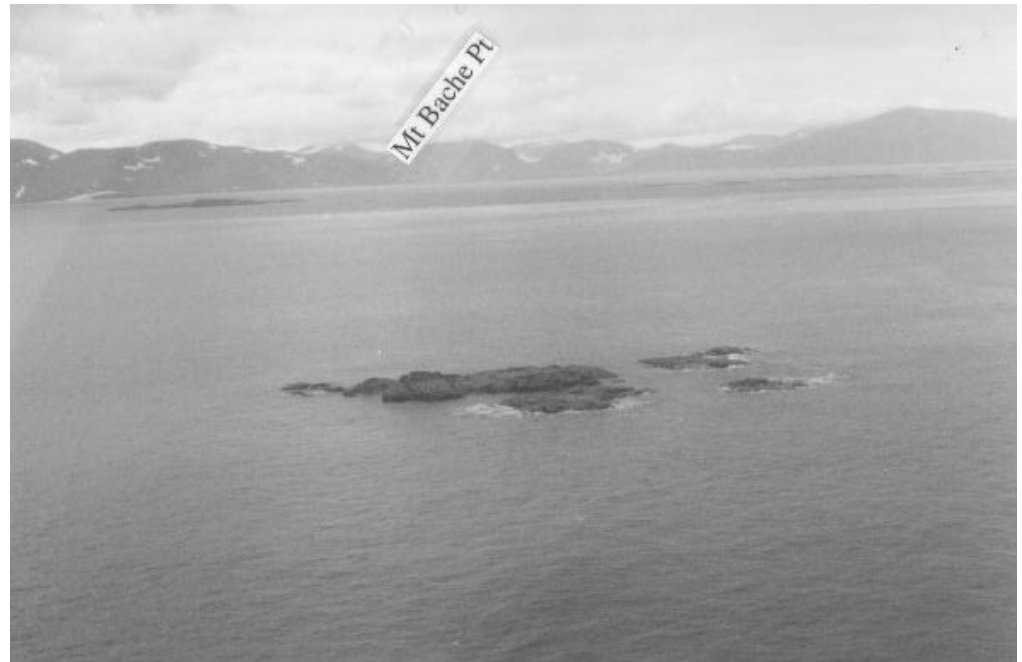
Figure 9. Unnamed rock on the east side of the Galvano Group. The rock was spotted in airphotos. The GPS position of the rock is 59° 55' 30"N, 63° 52' 55"W, which is about 430m north of the uncontrolled airphoto mosaic position. The rock is 0.5m above high water. Note the common islands in the middle distance 'moving' relative to the hills in the background of Figures 8 and 9.
