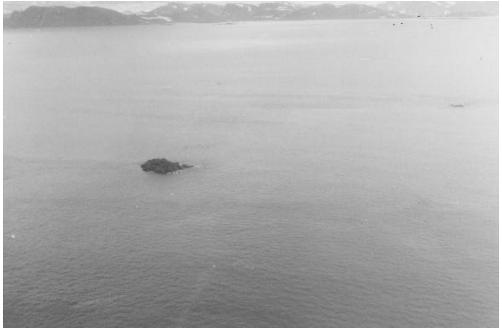
Figure 16. Landsat Island. The rock was spotted in satellite imagery in 1973, positioned in 1976 by sextant resection angles between distant hill tops. The GPS position of the island is 60^{\circ} 10' 37''\text{N} , 64^{\circ} 02' 30''\text{W} , and is 6.6m above high water. The GPS position is 70m east of the resection position. The rock, to the north was not seen in the 1973 imagery, the 1976 field work, nor the 1996 airphoto analysis but only during the 1997 survey. Even then, it was only because the survey was done at low tide. Its GPS position is 60^{\circ} 10' 47''\text{N} , 64^{\circ} 02' 36''\text{W} , and its height is 0.8m above low water.
