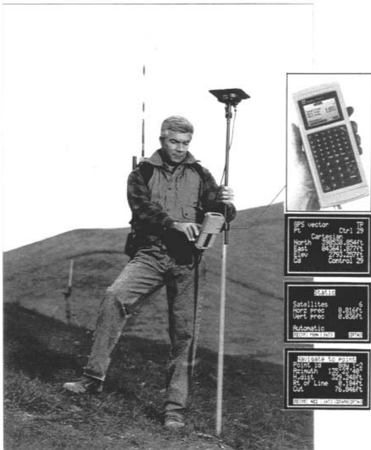
Figure 18: A Portable GPS Receiver with the Antenna and Controller (Courtesy of Trimble Navigation).
